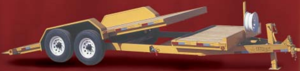
16' x 4' Tilt Bed with Stationary Front
